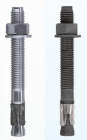
ICCONS® THRU-BOLT™ PRO is a pre-assembled torque controlled mechanical stud anchor, which when tightened draws the tapered end of the bolt into the expander clip expanding it to create expansion forces against the wall of the hole.
