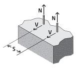
Note: To achieve 100% anchor capacity, critical spacing (S<sub>cr</sub>) is equal to 2 x h<sub>embed</sub>. Minimum spacing (S<sub>min</sub>) is equal to h<sub>embed</sub> at which the anchor achieves 50% of capacity.
