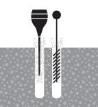
Blow and clean Clean the drill hole completely of dust and debris. Use blow pump and brush
