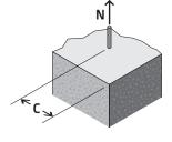
Note: To achieve 100% anchor capacity, critical edge distance (C<sub>cr</sub>) is equal to 12d (12 x anchor diameter). Minimum edge distance (C<sub>min</sub>) is equal to (5d) at which the anchor achieves 75% of capacity.
