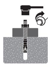
4. Apply torque Apply nominal installation torque using a torque wrench. Once installed verification of the total length of the anchor can be made through the letter on the head.
