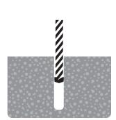
1. Drilling Use drill in hammer mode. Drill to specified diameter and depth for the required size.
