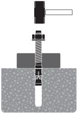
3. Install Insert the anchor in the hole to the specified embedment depth. Use hammer if required; DOMTA tool can be used alternatively. The installation may be done through the fixture baseplate.
